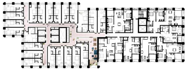
Image 4: typical proposed floor plan (co-living on the left, C3 residential on the right)
